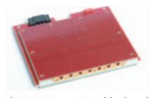
The SW0425-8 is a 1P8T wideband switch module with low loss and high resolution. It operates in the  $380~\mathrm{MHz}$  to  $2.5~\mathrm{GHz}$  frequen-
