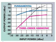
Fig. 5 Measured output power at 3 GHz and third harmonic power (IM3) vs. input power.
