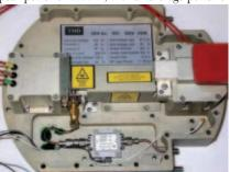
W for short periods. It operates at the top of the Ku radar band, at a high duty of up to 33 percent, and at very high pulse repetition frequency. The TWT is also equipped to work in a harsh environment.
