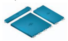
Pulsar Microwave Corp. introduces a new series of 0.5 to 8 GHz three-, four- and eight-way power dividers. All three models have 18 dB isolation and the insertion losses for the three-, four- and eight-way power dividers are 1.5, 1.8 and 2.6 dB, respectively.
